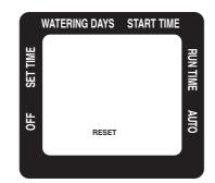
Press and hold for 5 seconds to erase all settings in the timer and it will return to the original factory settings. The screen will display RESET.
