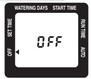
'OFF' mode is used to stop watering for an extended period of time. Press ② untill the arrow is pointed to 'OFF'.
