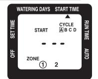
'Start Time' is the time of day that the tap timer will begin watering. You can set up to 4 cycles (start times) per zone.
