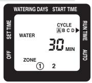
'Run Time' sets the length of time that the cycle will water for. You can set a different run time per cycle per zone.
