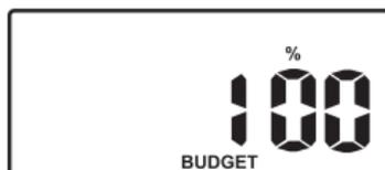
Displayed is the word “*Budget*” and “100%”. This represents the current automatic watering run times as being 100%. The percentage budget can be set in 25% increments from 25% up to 150%.
