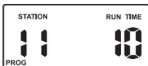
This means station 1 has a default run time of 10 minutes in program 1. “Station 1” will be flashing.
