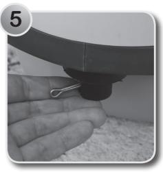
Take your Auto Rewind Hose Reel, and remove the securing pin at the base of the mounting tube. Remove the mounting tube from the hose reel and slot the hose reel inside the wall bracket, so the fitting tube hole lines up with the wall bracket hole. Then replace the mounting tube into its hole to hold the hose reel in place and replace the securing pin into the base of the mounting tube.
