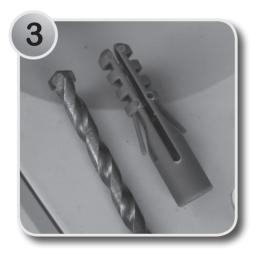
Take the wall plugs (supplied with the hose reel) and measure the correct drill bit width to use.
