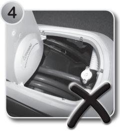
Locking bars in the **WRONG** position. The bars will catch on the reel & prevent it from working correctly.
