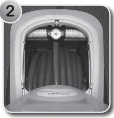
If the hose isn't extending properly, this may be caused by the screws securing the guide hole being too tight.
