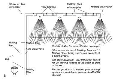
Work out the spacing of the misting jets and cut the misting hose to length and install the relevant misting tees. Finish each line with a misting elbow.
