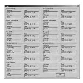
This section is used to display the recorded min and max value recorded with time stamp. Min/Max reset can only be done through key operation on the base station.
