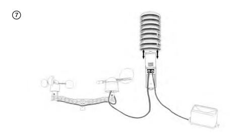
The rain sensor's cable is connected to the input marked Rain on the thermo-hygrosensor(see fig.7)
