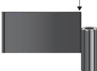
2) Slot the panels in the pillars with the tongue facing up.
